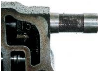
heavy deposit build-up.
