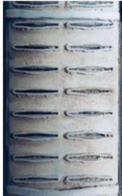
Rust, scale and sludge can plug cooling system fins, preventing proper circulation of coolant.
